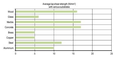
The tests have been conducted at 20°C on metal to metal joints, which have been hardened for 48 hours at 20°C.
